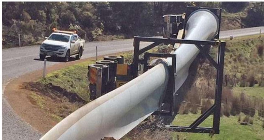
Figure 5-2: Wind turbine blade transport rollover (Source: Tasmanian Police)
