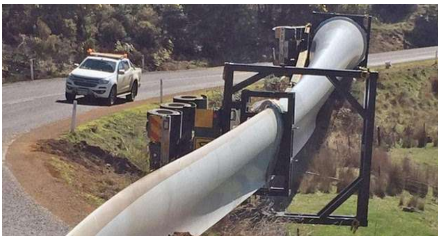
Figure 5-2: Wind turbine blade transport rollover (Source: Tasmanian Police)
