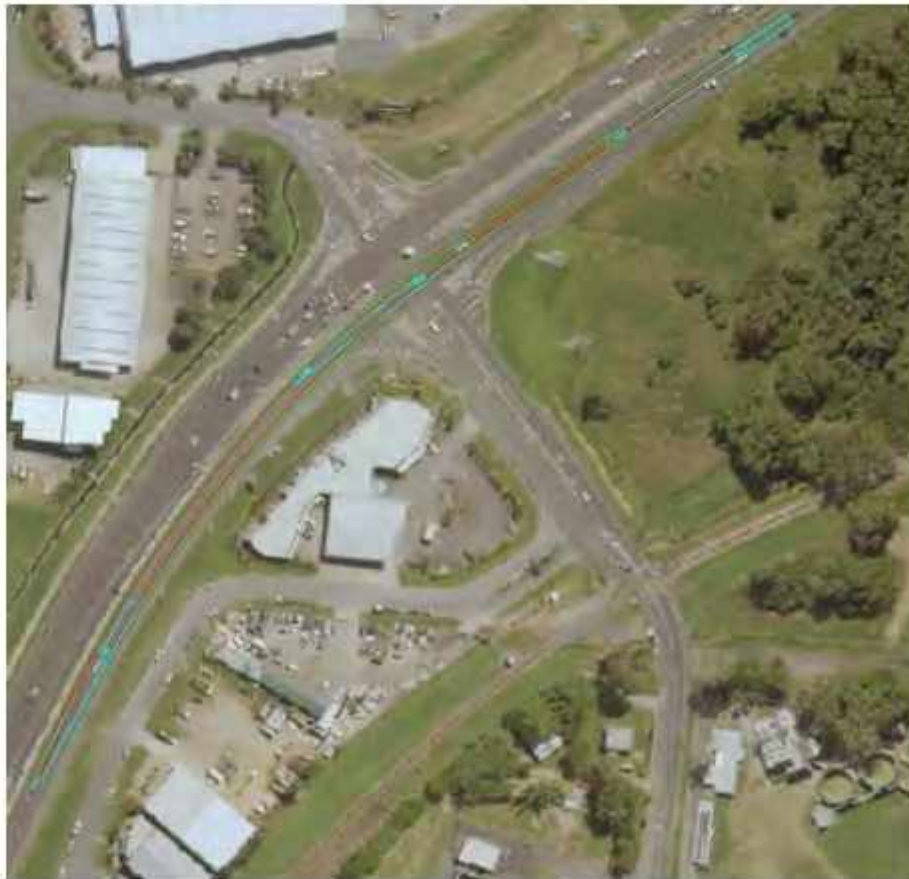
Figure 15 Swept Path Pinch Point 4 with 83.5m Blade
