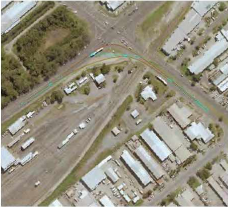
Figure 14 Swept Path Pinch Point 3 with 83.5m Blade
