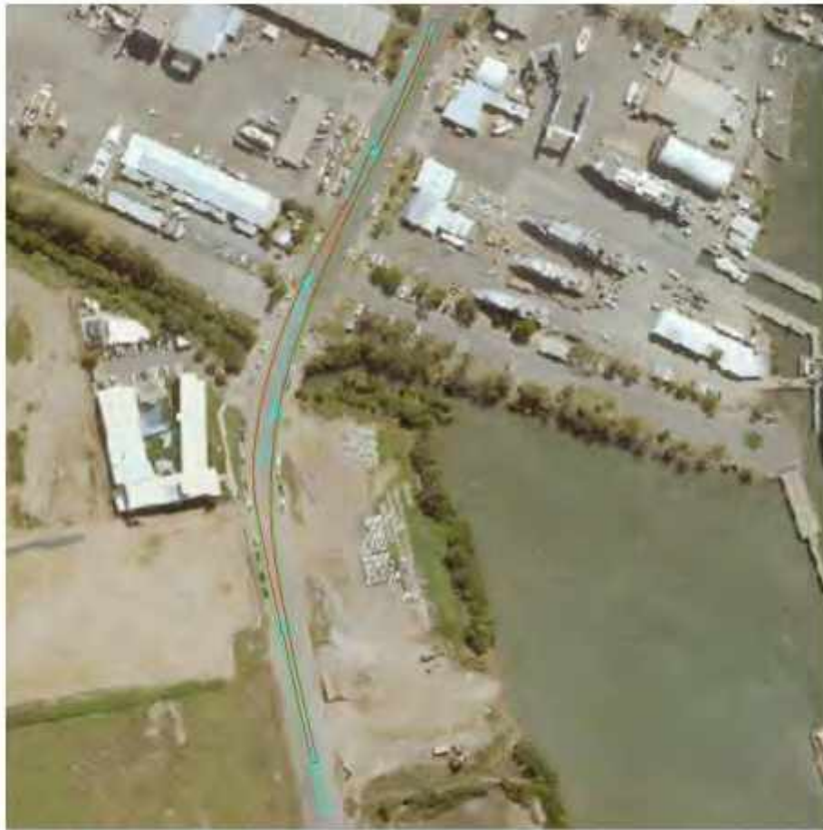
Figure 12 Swept Path Pinch Point 1 with 83.5m Blade
