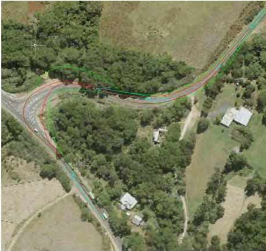
Figure 33 Swept Path Pinch Point 23 with 93.5m Blade
