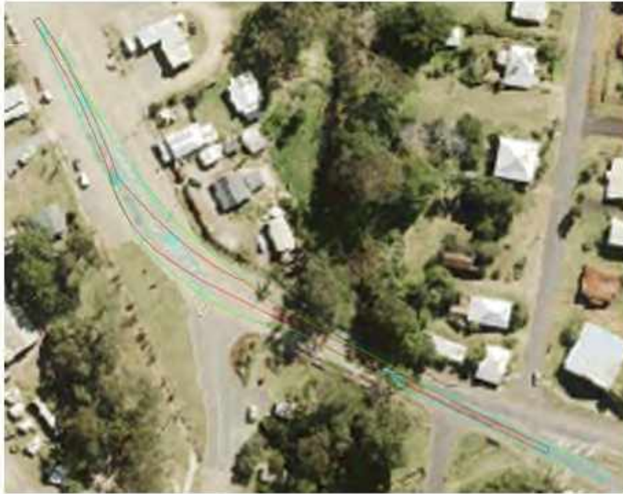
Figure 35 Swept Path Pinch Point 25 with 83.5m Blade
