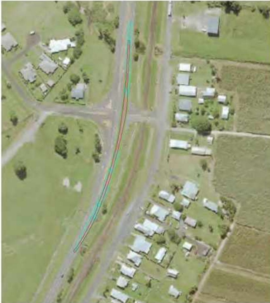
Figure 17 Swept Path Pinch Point 6 with 83.5m Blade
