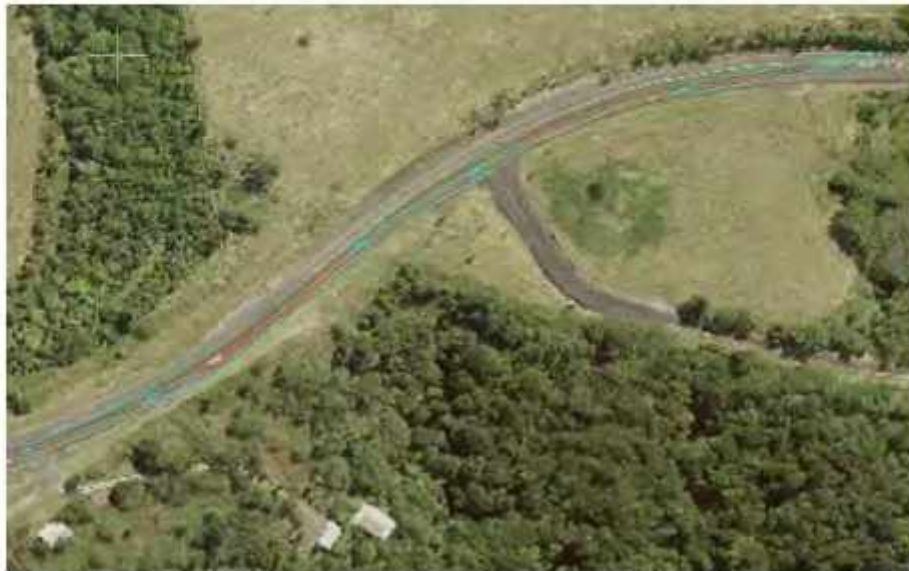
Figure 30 Swept Path Pinch Point 20 with 83.5m Blade
