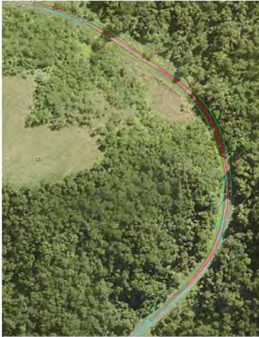
Figure 27 Swept Path Pinch Point 17 with 83.5m Blade
