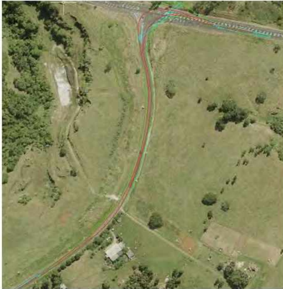
Figure 29 Swept Path Pinch Point 19 with 83.5m Blade
