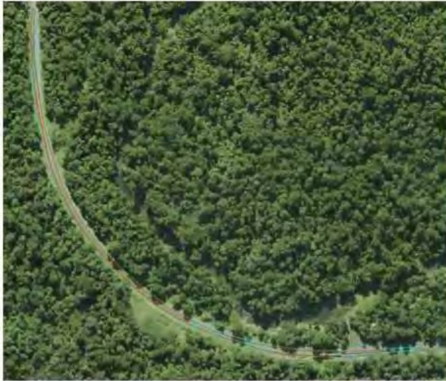
Figure 23 Swept Path Pinch Point 13 with 83.5m Blade
