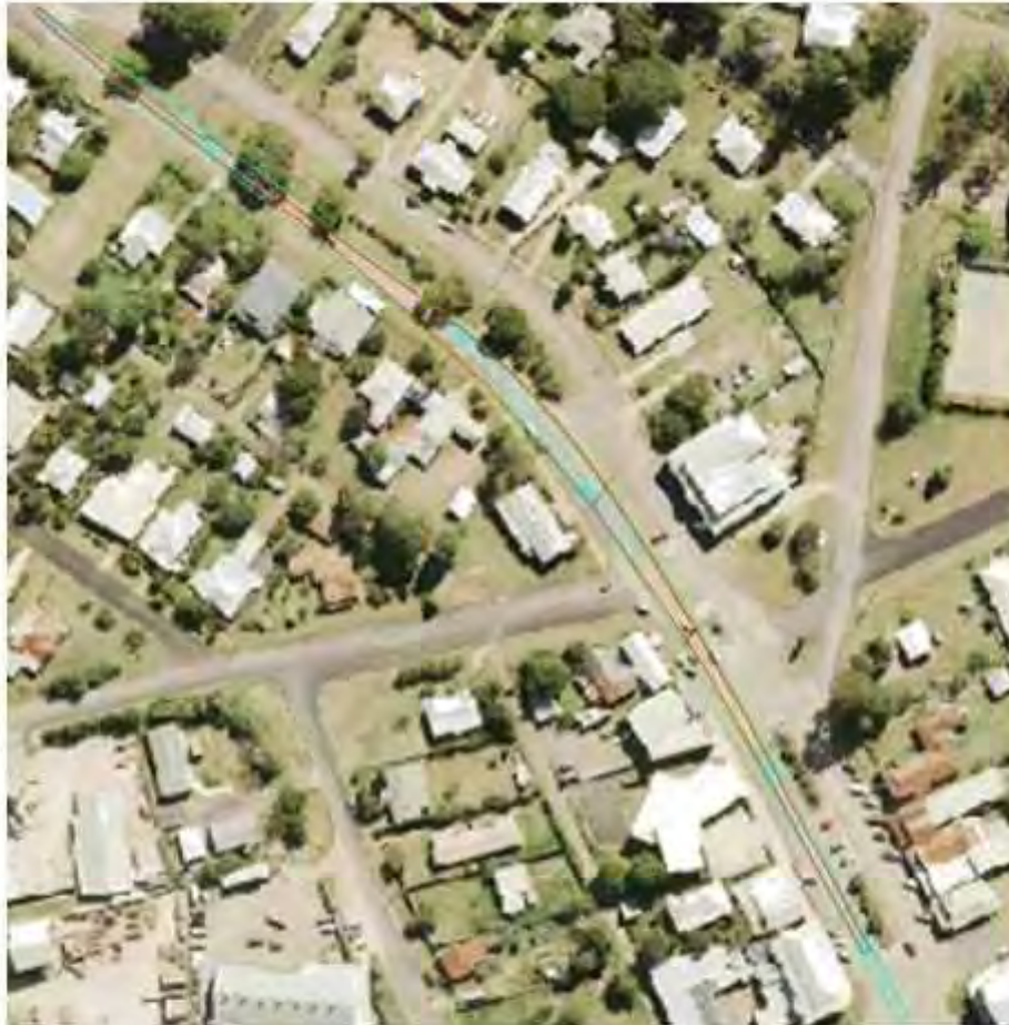
Figure 36 Swept Path Pinch Point 20 with 83.5m Blade
