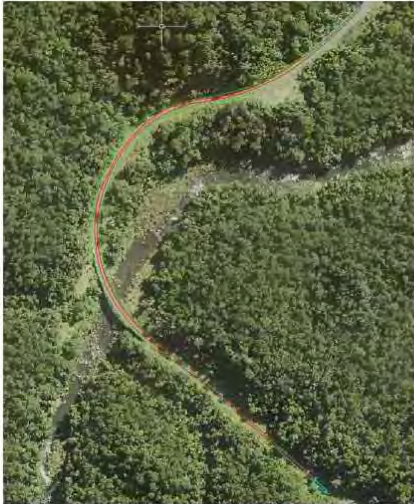
Figure 26 Swept Path Pinch Point 16 with 83.5m Blade
