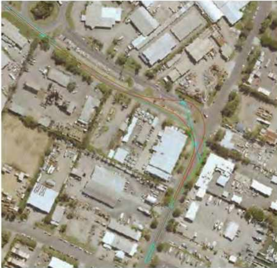
Figure 13 Swept Path Pinch Point 2 with 83.5m Blade
