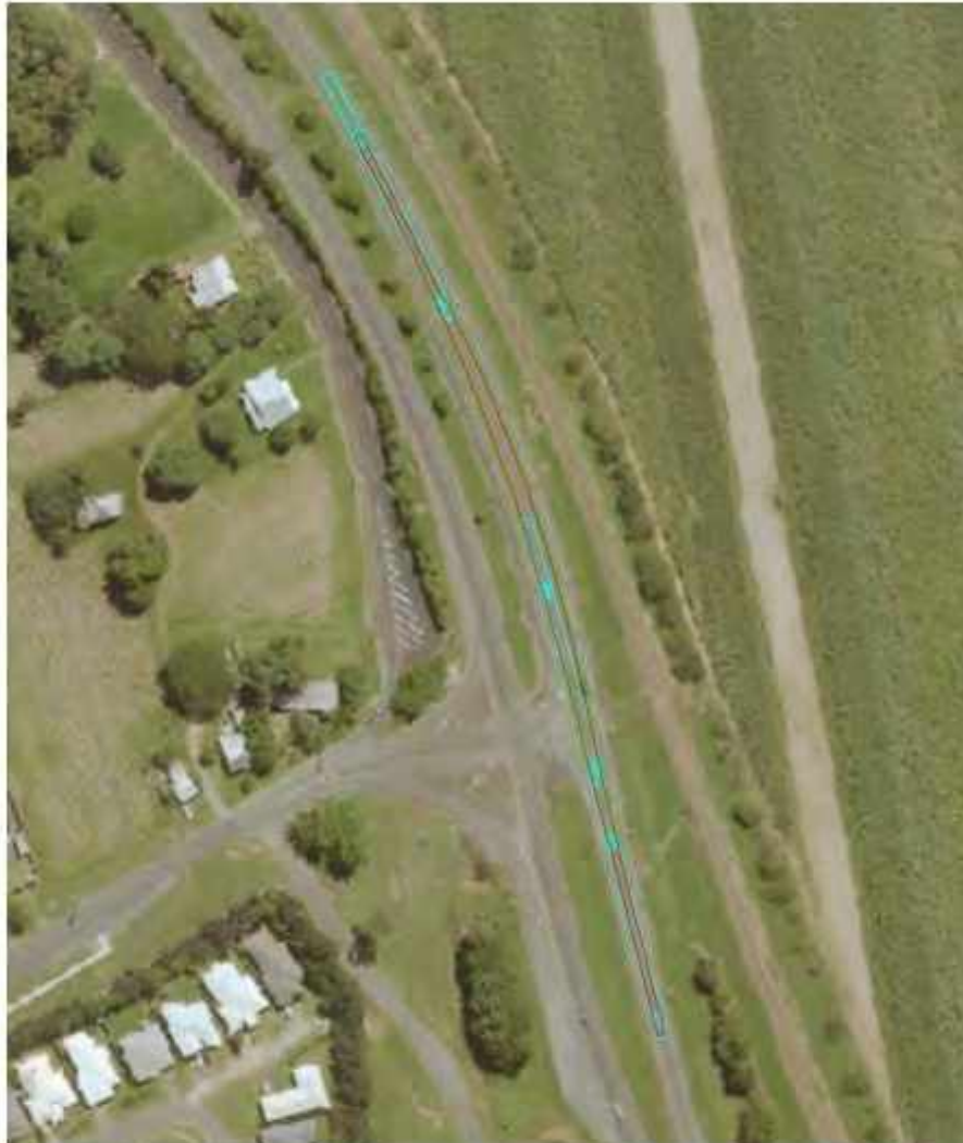
Figure 16 Swept Path Pinch Point 5 with 83.5m Blade
