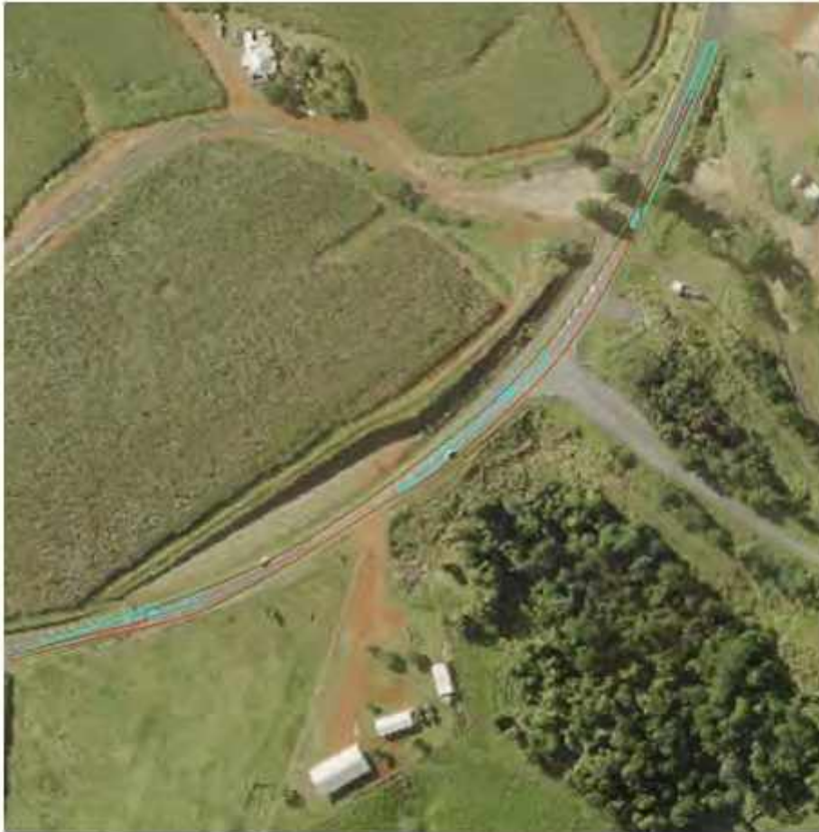
Figure 20 Swept Path Pinch Point 10 with 83.5m Blade
