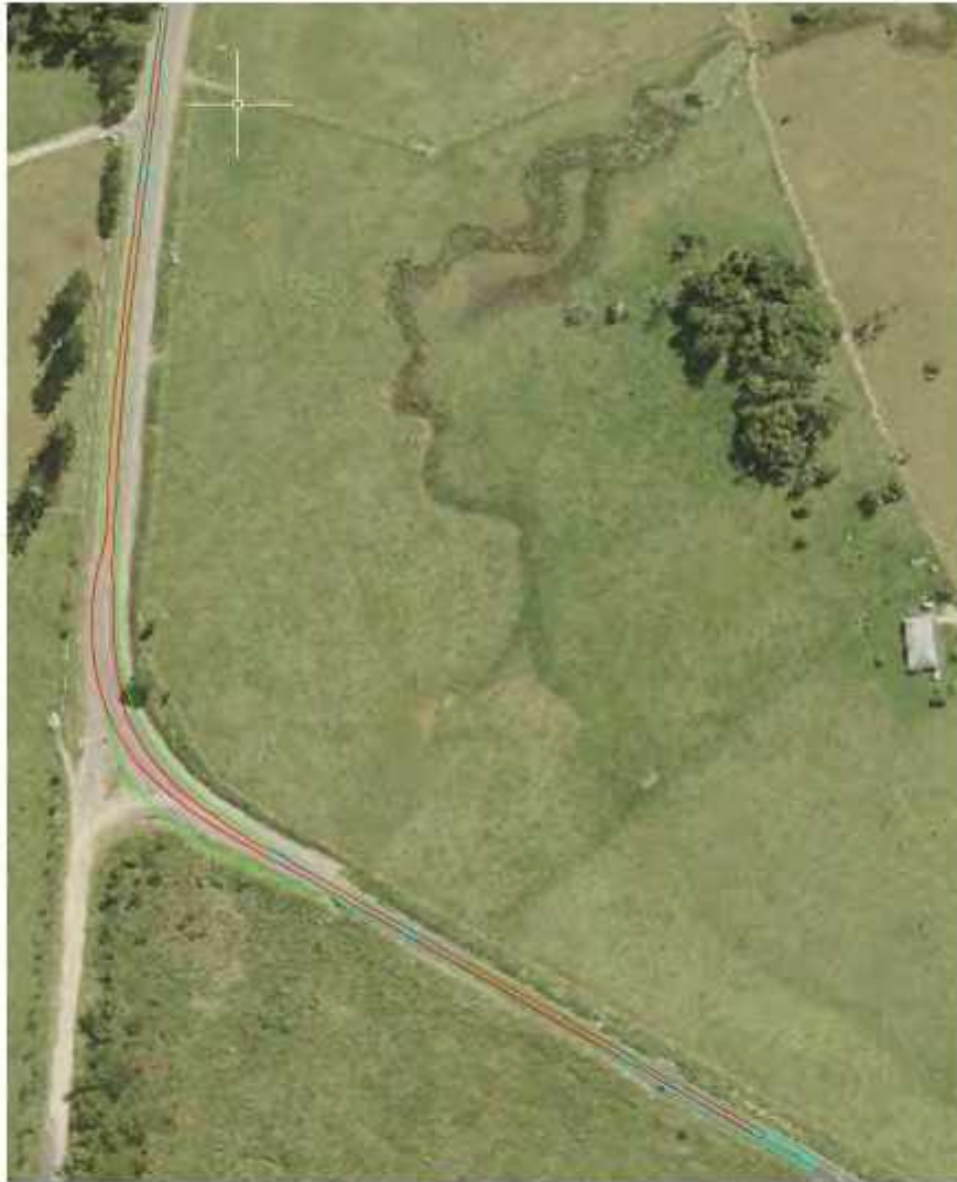
Figure 31 Swept Path Pinch Point 21 with 83.5m Blade
