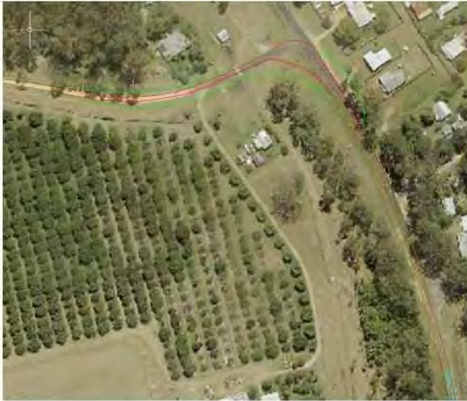
Figure 38 Swept Path Pinch Point 28 with 83.5m Blade
