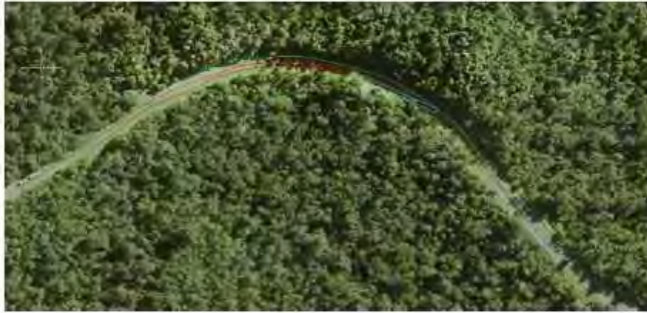
Figure 25 Swept Path Pinch Point 15 with 83.5m Blade
