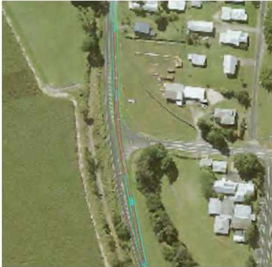
Figure 18 Swept Path Pinch Point 7 with 83.5m Blade
