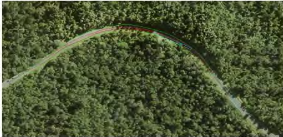
Figure 25 Swept Path Pinch Point 15 with 83.5m Blade
