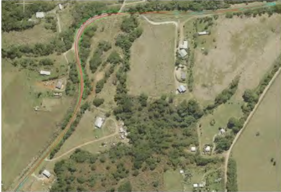
Figure 32 Swept Path Pinch Point 22 with 83.5m Blade
