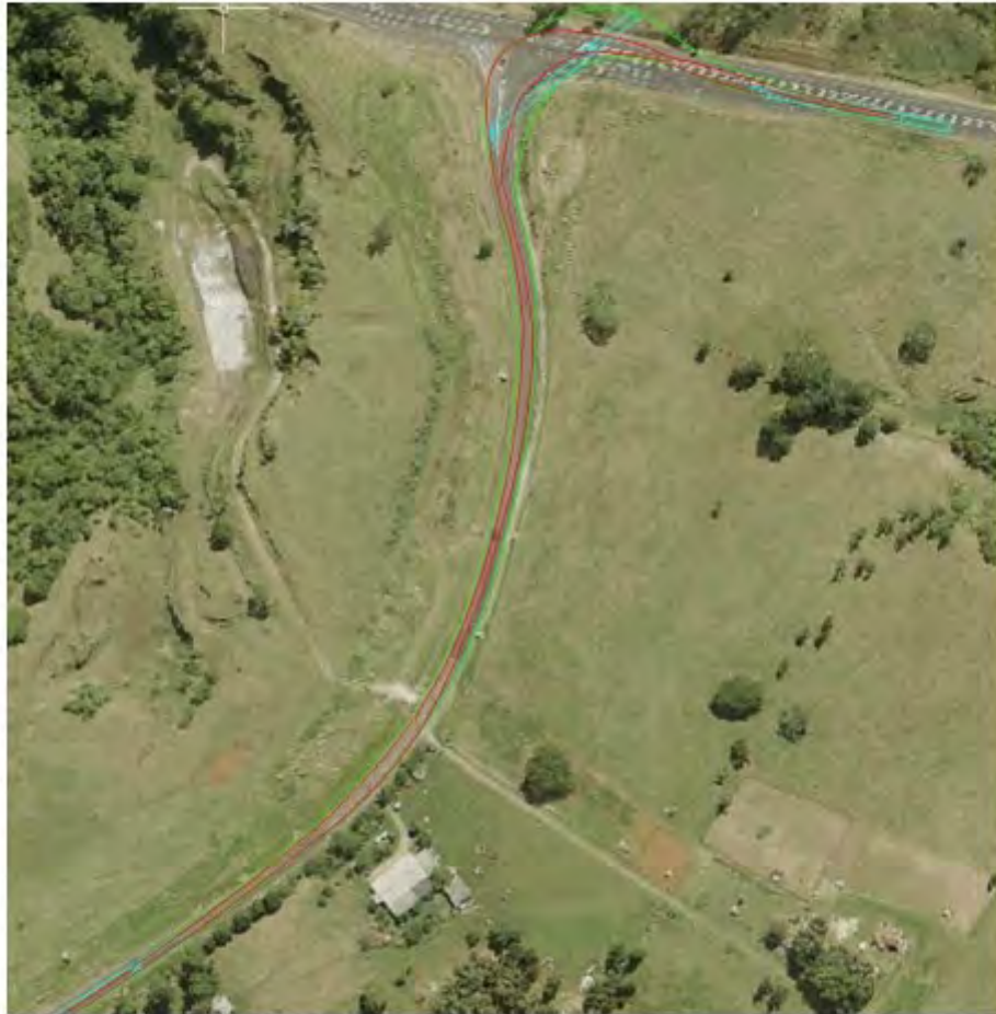
Figure 29 Swept Path Pinch Point 19 with 83.5m Blade
