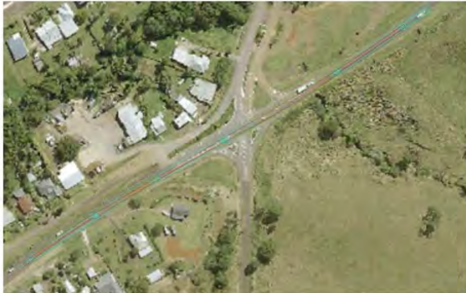
Figure 28 Swept Path Pinch Point 18 with 83.5m Blade
