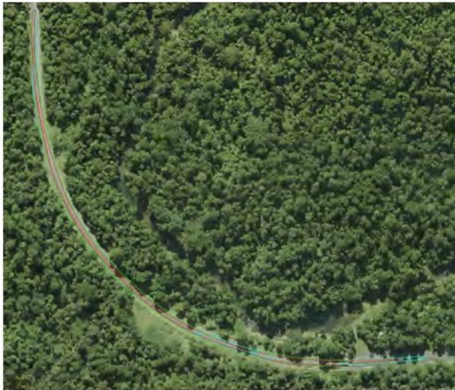
Figure 23 Swept Path Pinch Point 13 with 83.5m Blade
