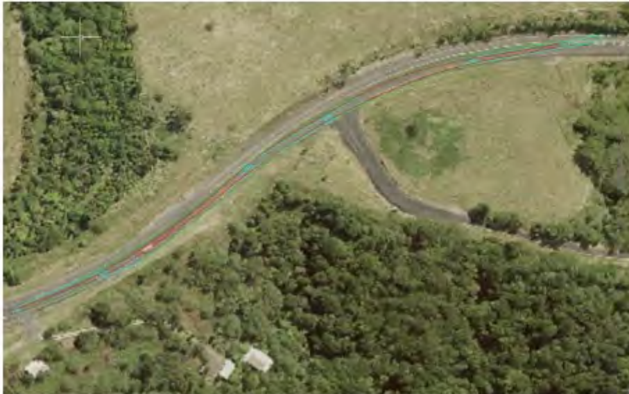
Figure 30 Swept Path Pinch Point 20 with 83.5m Blade
