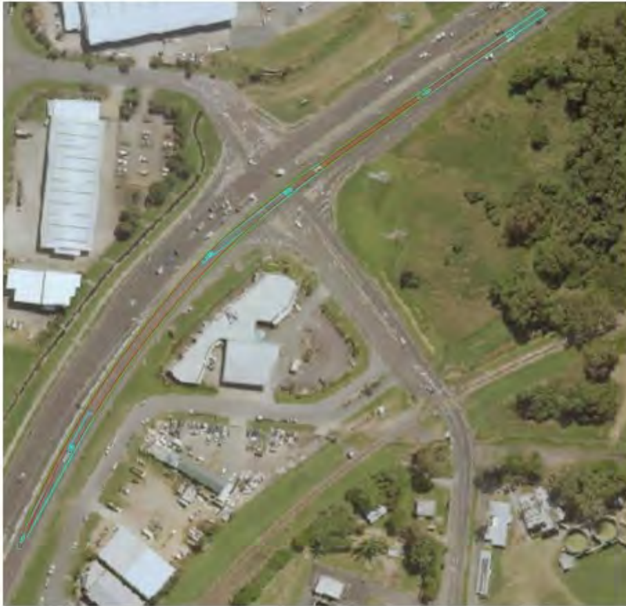
Figure 15 Swept Path Pinch Point 4 with 83.5m Blade
