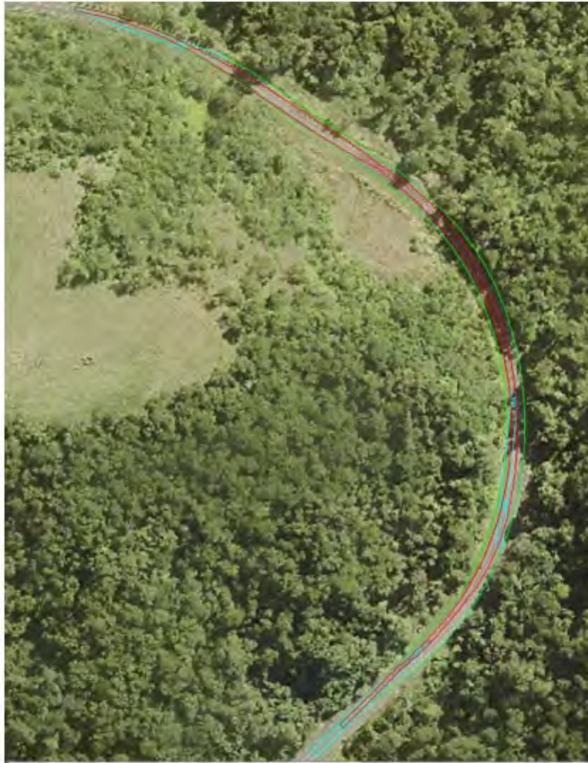
Figure 27 Swept Path Pinch Point 17 with 83.5m Blade
