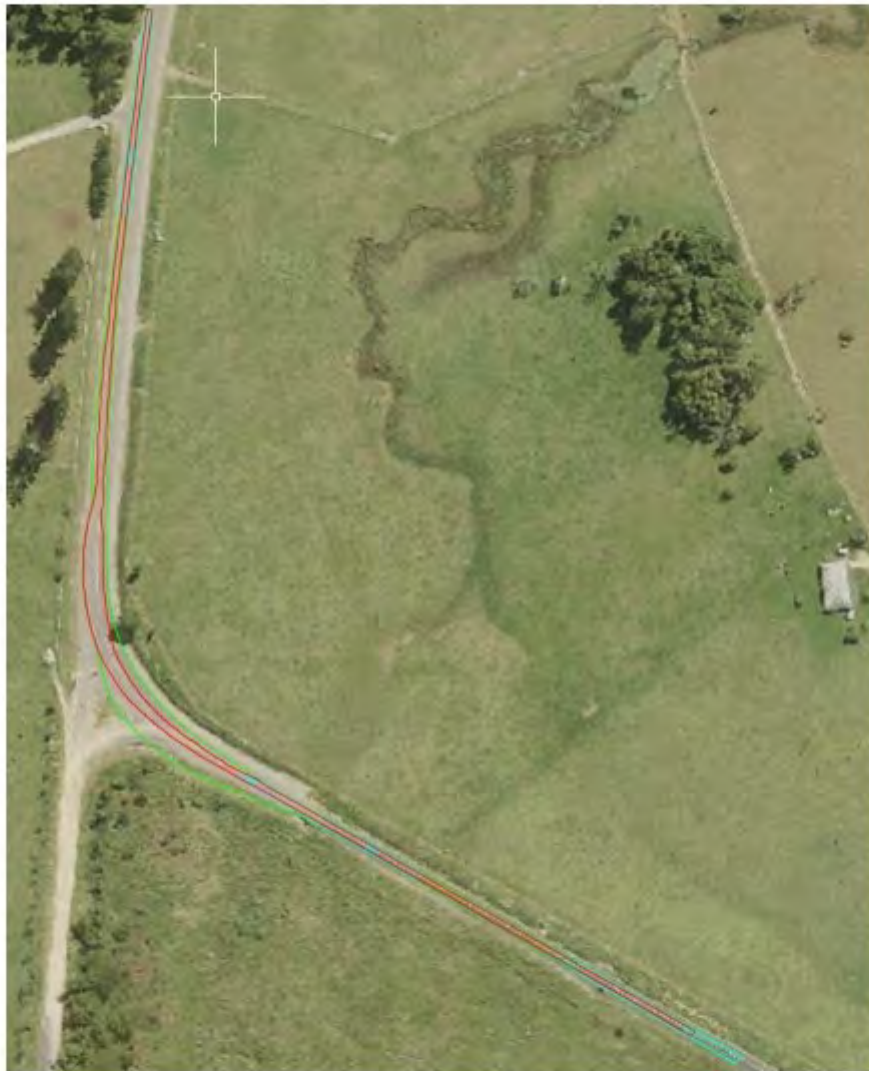
Figure 31 Swept Path Pinch Point 21 with 83.5m Blade
