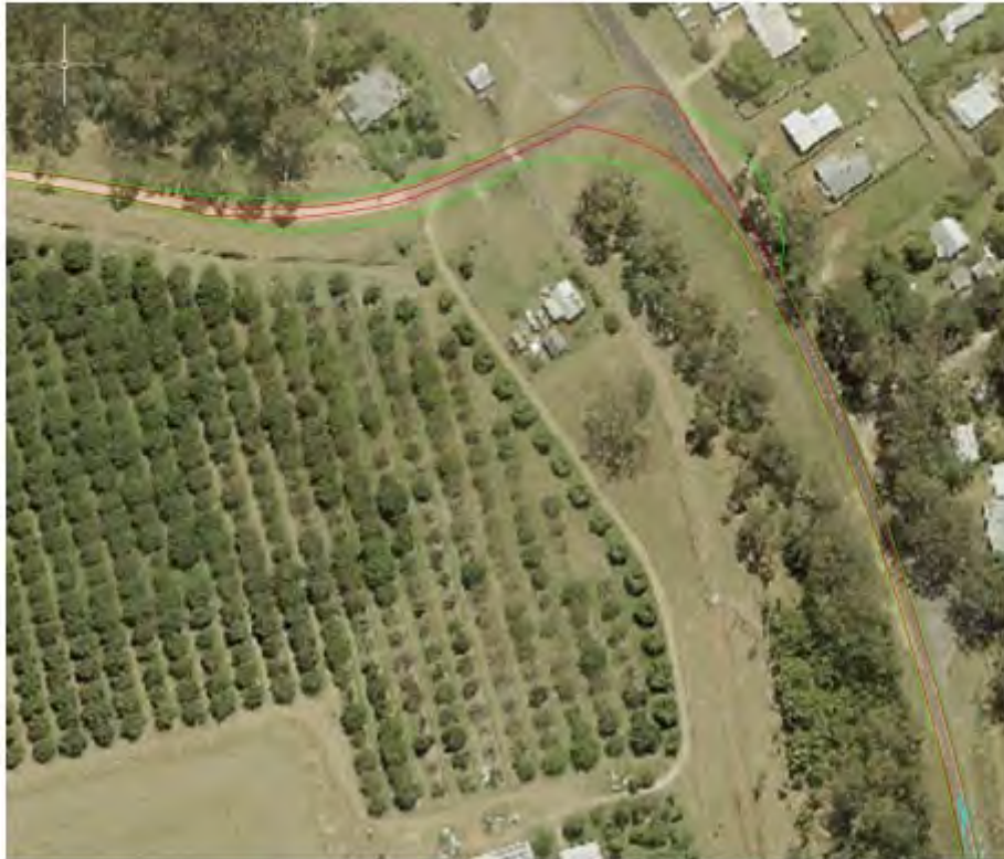
Figure 38 Swept Path Pinch Point 28 with 83.5m Blade
