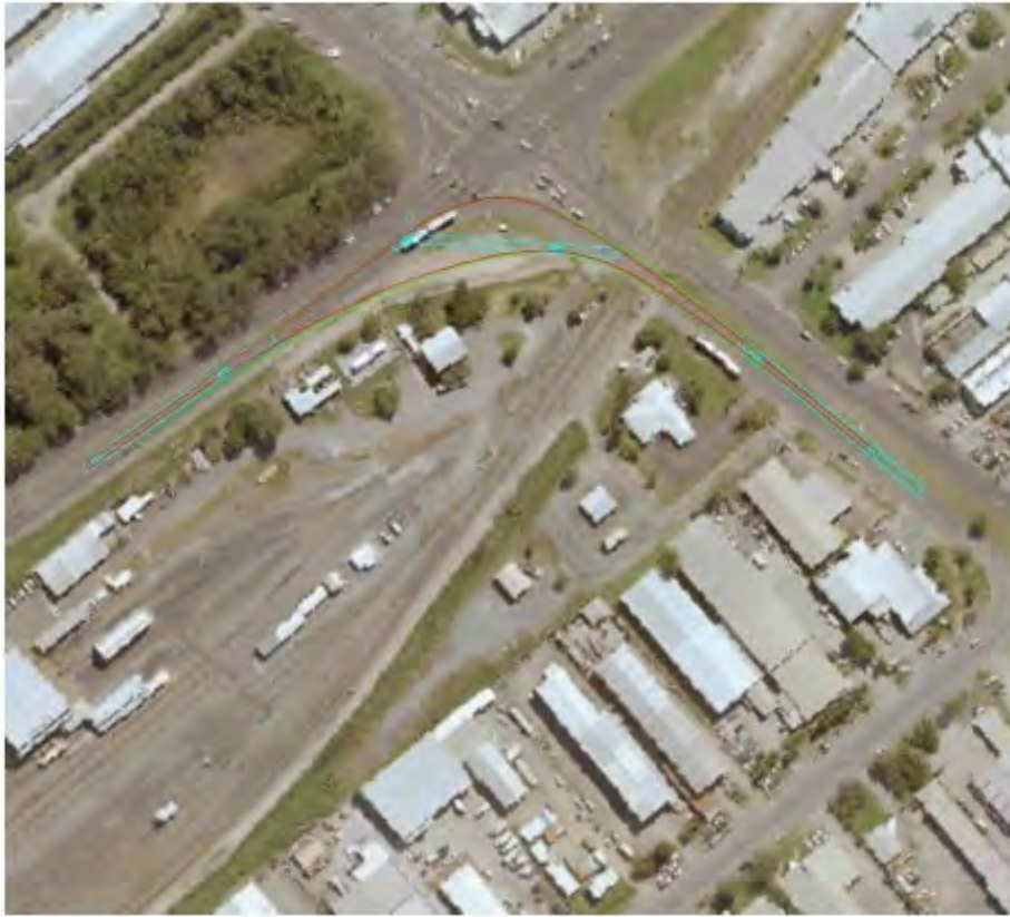
Figure 14 Swept Path Pinch Point 3 with 83.5m Blade
