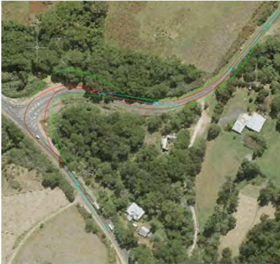
Figure 33 Swept Path Pinch Point 23 with 83.5m Blade
