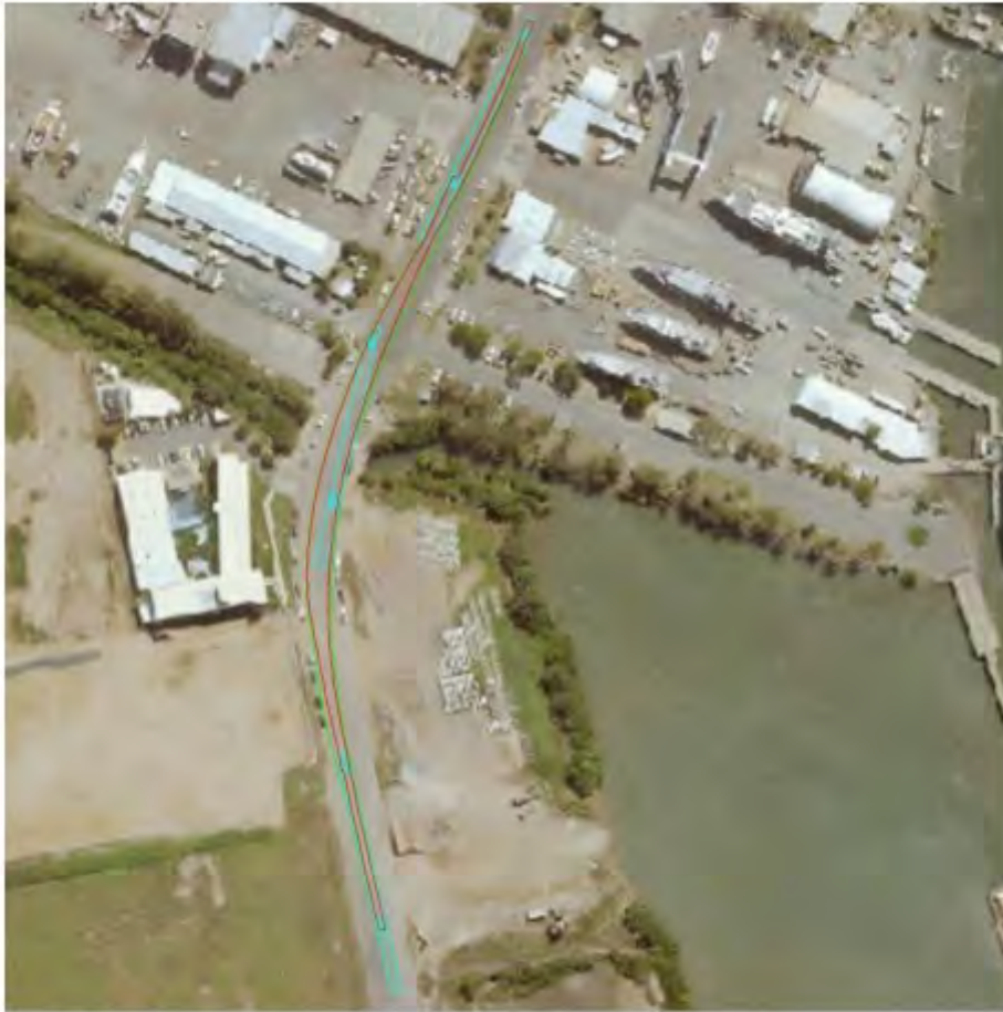
Figure 12 Swept Path Pinch Point 1 with 83.5m Blade
