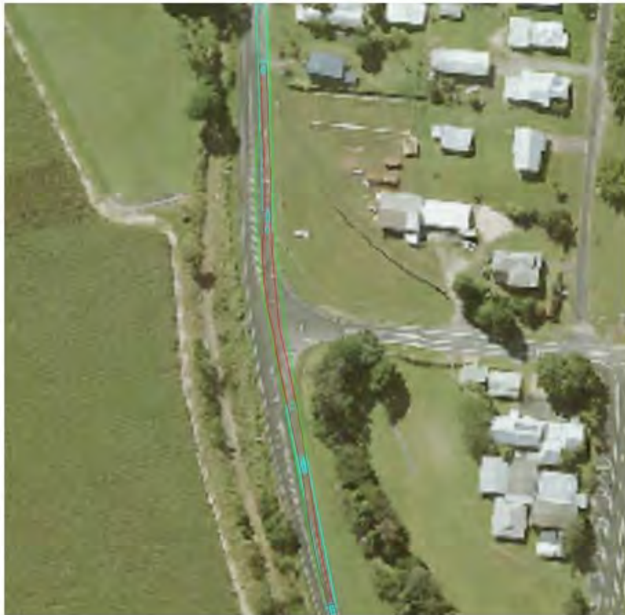
Figure 18 Swept Path Pinch Point 7 with 83.5m Blade
