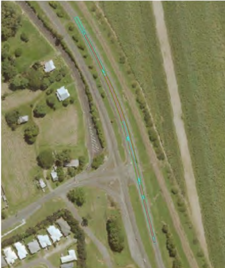
Figure 16 Swept Path Pinch Point 5 with 83.5m Blade
