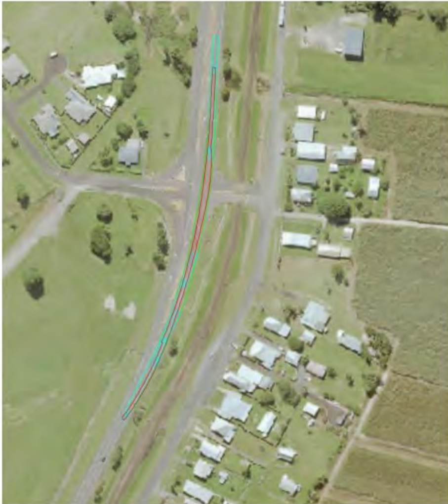
Figure 17 Swept Path Pinch Point 6 with 83.5m Blade
