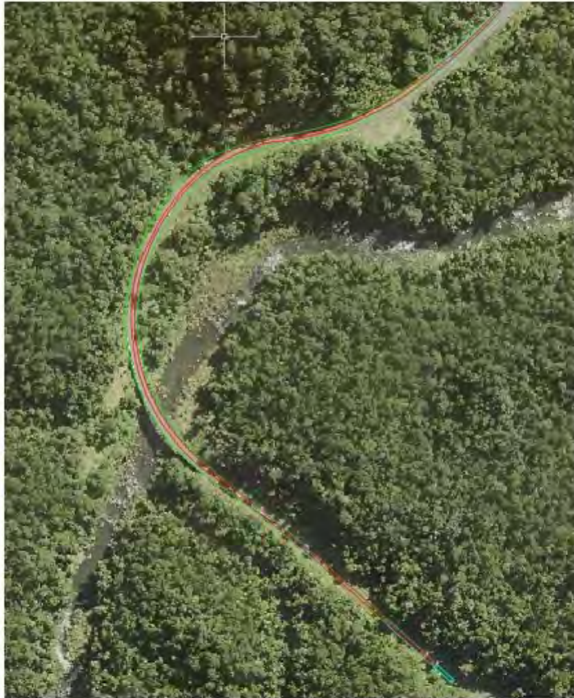
Figure 26 Swept Path Pinch Point 16 with 83.5m Blade
