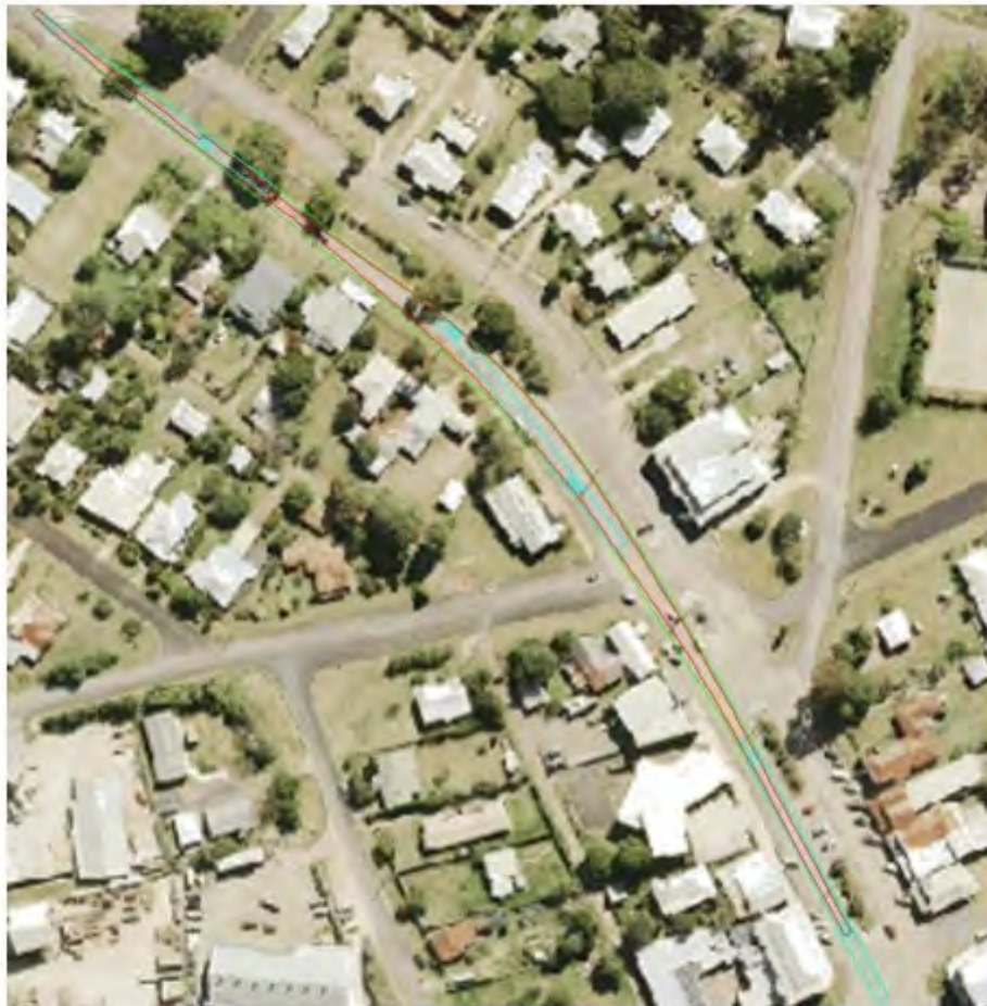
Figure 36 Swept Path Pinch Point 26 with 83.5m Blade
