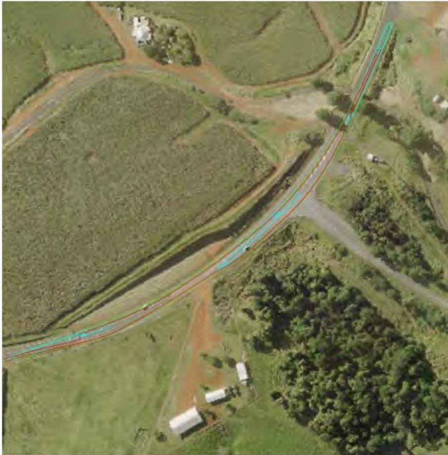
Figure 20 Swept Path Pinch Point 10 with 83.5m Blade
