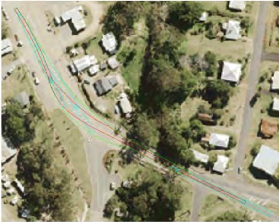
Figure 35 Swept Path Pinch Point 25 with 83.5m Blade
