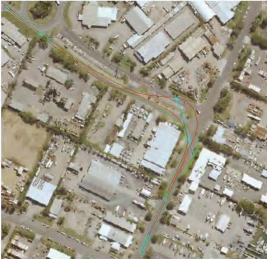
Figure 13 Swept Path Pinch Point 2 with 83.5m Blade
