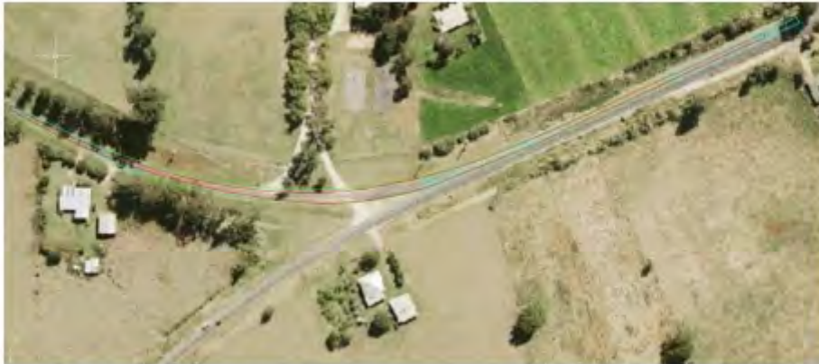
Figure 34 Swept Path Pinch Point 24 with 83.5m Blade
