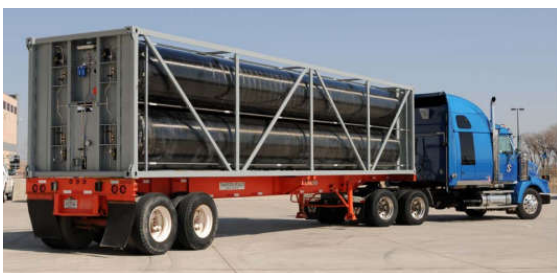
Figure 3: Type IV composite (257bar) tube skid on trailer Source: Lincoln Composites
