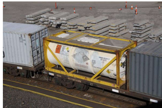
Figure 5: 20' ISO tanktainer on rail skid wagon Source: Wongm's Rail Gallery
