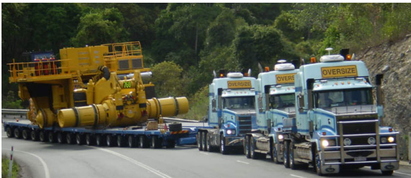
Figure 7.11: 165 TONNE OSOM UP THE ETON RANGE ON PEAK DOWNS HIGHWAY
